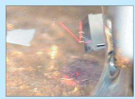
In-fluid observation when a cover glass is attached to the cantilever.
