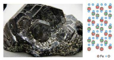
Appearance of hematite (α-Fe2O3) crystal, and schematic diagram of atomic structure and Fe atom magnetic moment(arrow) at room temperature.
