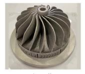
Impeller (Material: Nickel-based superalloy 718)
