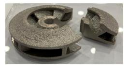
Impeller with shroud (Material: Nickel-based superalloy 718))
