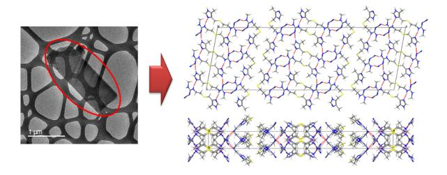
Figure: TEM image of cimetidine form B and crystalline structure solved by electron and NMR nano-crystallography. The cimetidine form B is needle shape crystals (indicated by red circle on the left figure) and often fails to form a large single crystal for single crystal X-ray diffraction. In addition, the contamination of form C is often observed, hampering the structural solution by powder X-ray diffraction. Here, we solved the crystalline structure of cimetidine form B for the first time.
